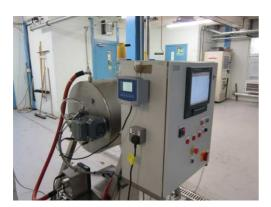
Crucially for process development and pilot work, a data recorder charts a range of Biomixer parameters including power consumption, pH, temperature and shaft rotation speed. This inline monitoring provides invaluable information for process optimisation in relation to substrate characteristics over time and overall energy efficiency. Moreover, the plug and play nature of the Biomixer design allows for new probes to be installed and their outputs recorded with a minimum of down time.
